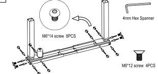
4 Overturn frame and attach brackets to beam using 4 of M6\*12 screws, and then fir the rubber cushions to the brackets and beams
