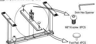
5 Loosen nut on each end of the transmission rod using spanner,connect the hex rod of the main leg to one end of the transmission rod and the hex rod of the transmission rod insert into the other leg
