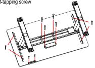
Attach legs to the beam using 8 of M6\*14 screws and 4 of M6\*12 screws
