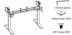
6 Overturn frame put on the table, distance from frame to table should be keep the same (usually5-8cm) tighten the screws on the beam and transmission rod
