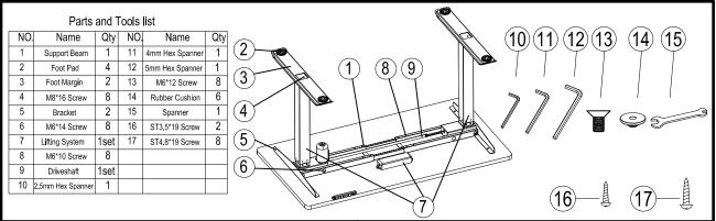
Loosen the 4 screws of beam using 4MM hex spanner, adjust the beam to proper position to fit the desktop
